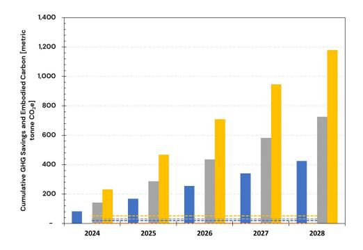
Figure A. 32: Embodied Carbon and Cumulative GHG Savings Over 5 Years (2024–2028) Using High RE Cost Electricity Emission Rates for CZ5 – Scenario 1: Natural Gas Heating
