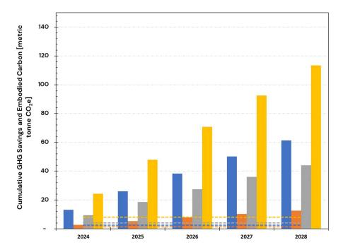
Figure A. 10: Embodied Carbon and Cumulative GHG Savings Over 5 Years (2024–2028) Using Medium RE Cost Electricity Emission Rates for CZ5 – Scenario 1: Current Heating Systems Mix
