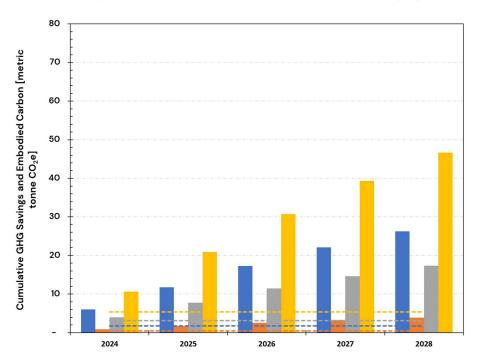
Figure A. 18: Embodied Carbon and Cumulative GHG Savings Over 5 Years (2024–2028) Using Low RE Cost Electricity Emission Rates for CZ3 – Scenario 2: 100% Heat Pump Systems
