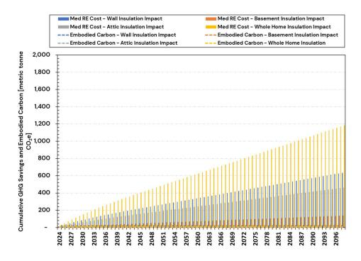
Figure A. 9: Embodied Carbon and Cumulative GHG Savings Over 75 Years (2024–2098) Using Medium RE Cost Electricity Emission Rates for CZ5 – Scenario 1: Current Heating Systems Mix
