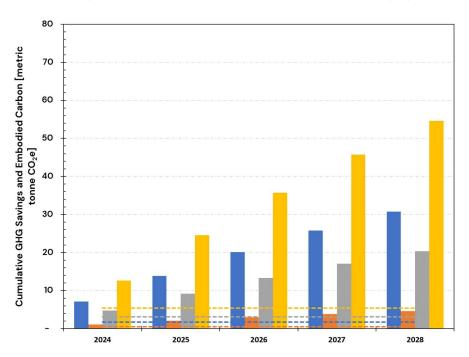
Figure A. 16: Embodied Carbon and Cumulative GHG Savings Over 5 Years (2024–2028) Using Medium RE Cost Electricity Emission Rates for CZ3 – Scenario 2: 100% Heat Pump Systems
