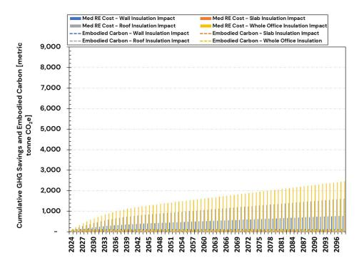
Figure A. 45: Embodied Carbon and Cumulative GHG Savings Over 75 Years (2024–2098) Using Medium RE Cost Electricity Emission Rates for CZ5 – Scenario 2: 100% Heat Pump Systems
