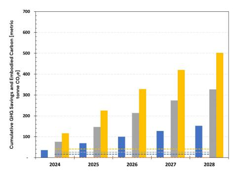
Figure A. 28: Embodied Carbon and Cumulative GHG Savings Over 5 Years (2024–2028) Using Medium RE Cost Electricity Emission Rates for CZ3 – Scenario 1: Natural Gas Heating
