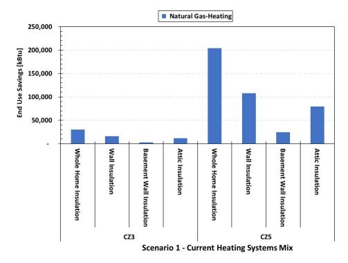
Figure 4: Impact of Insulation on Natural Gas End Use Savings for the Case with the Current Heating Systems Mix
