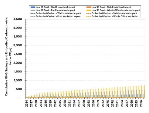
Figure A. 41: Embodied Carbon and Cumulative GHG Savings Over 75 Years (2024–2098) Using Low RE Cost Electricity Emission Rates for CZ3 – Scenario 2: 100% Heat Pump Systems
