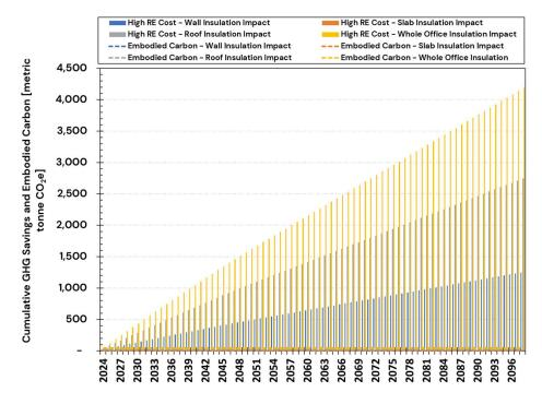
Figure A. 37: Embodied Carbon and Cumulative GHG Savings Over 75 Years (2024–2098) Using High RE Cost Electricity Emission Rates for CZ3 – Scenario 2: 100% Heat Pump Systems
