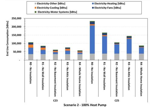
Figure 7: Electricity End Use Consumption for the Case with 100% Heat Pump Systems
