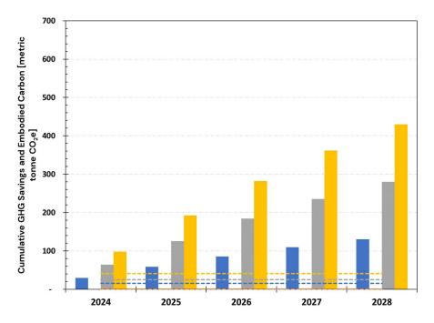
Figure A. 30: Embodied Carbon and Cumulative GHG Savings Over 5 Years (2024–2028) Using Low RE Cost Electricity Emission Rates for CZ3 – Scenario 1: Natural Gas Heating
