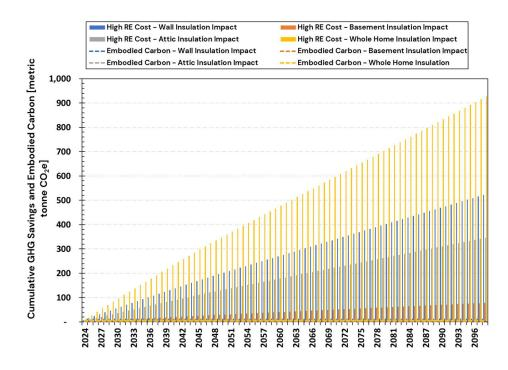
Figure A. 13: Embodied Carbon and Cumulative GHG Savings Over 75 Years (2024–2098) Using High RE Cost Electricity Emission Rates for CZ3 – Scenario 2: 100% Heat Pump Systems
