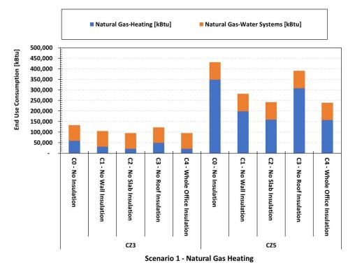
Figure 11: Natural Gas End Consumption for Scenario 1 – Natural Gas Heating
