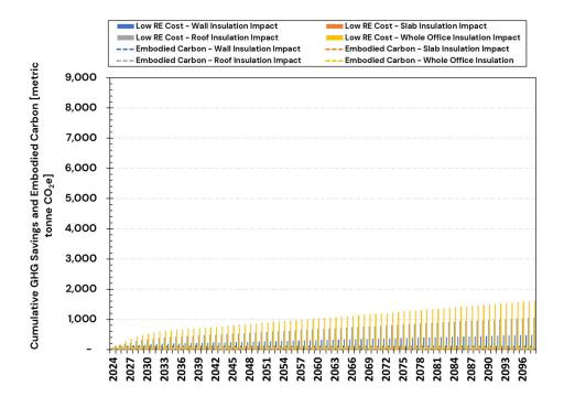
Figure A. 29: Embodied Carbon and Cumulative GHG Savings Over 75 Years (2024–2098) Using Low RE Cost Electricity Emission Rates for CZ3 – Scenario 1: Natural Gas Heating
