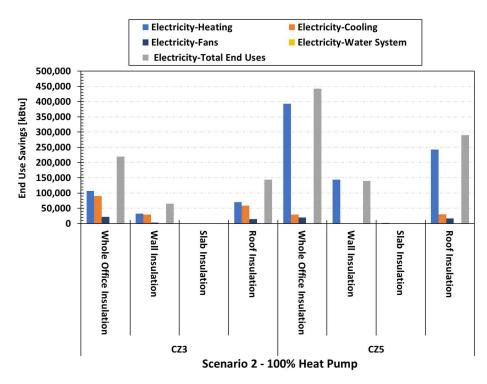
Figure 14: Impact of Insulation on Electricity End Use Percent Savings for the Case with 100% Heat Pump Systems (Commercial Prototype)
