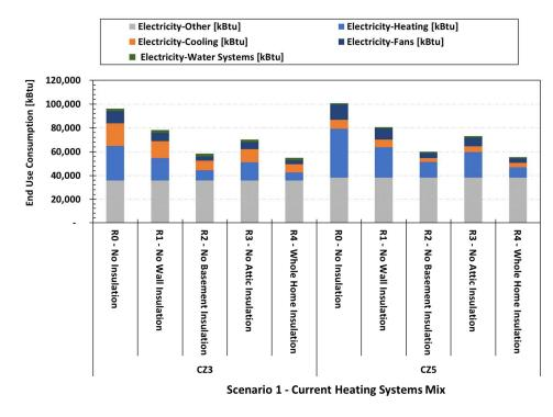
Figure 1: Electricity End Use Consumption for the Case with the Current Heating Systems Mix
