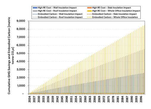
Figure A. 25: Embodied Carbon and Cumulative GHG Savings Over 75 Years (2024–2098) Using High RE Cost Electricity Emission Rates for CZ3 – Scenario 1: Natural Gas Heating
