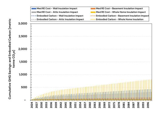
Figure A. 21: Embodied Carbon and Cumulative GHG Savings Over 75 Years (2024–2098) Using Medium RE Cost Electricity Emission Rates for CZ5 – Scenario 2: 100% Heat Pump Systems
