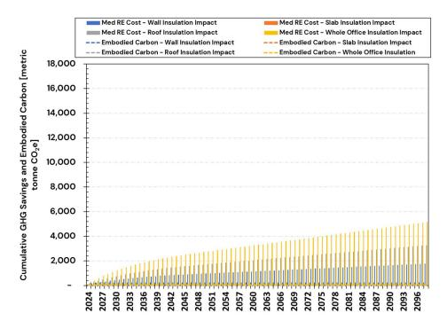
Figure A. 33: Embodied Carbon and Cumulative GHG Savings Over 75 Years (2024–2098) Using Medium RE Cost Electricity Emission Rates for CZ5 – Scenario 1: Natural Gas Heating
