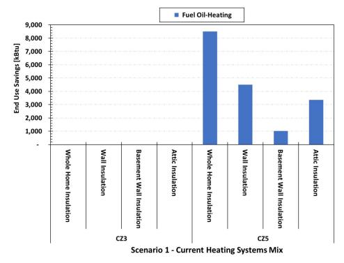
Figure 6: Impact of Insulation on Fuel Oil End Use Percent Savings for the Case with the Current Heating Systems Mix
