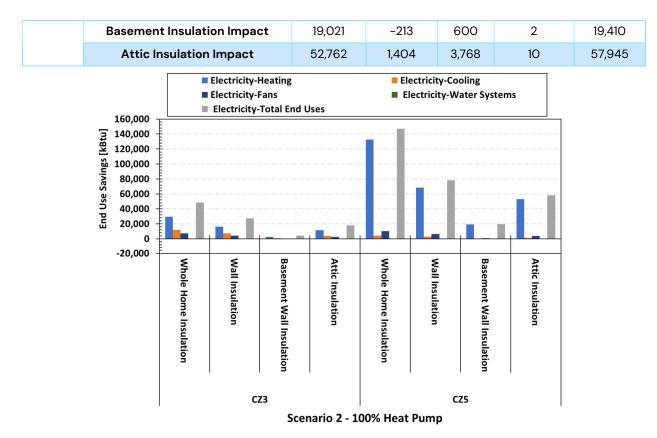
Figure 8: Impact of Insulation on Electricity End Use Savings for the Case with 100% Heat Pump Systems
