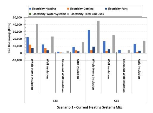
Figure 2: Impact of Insulation on Electricity End Use Savings for the Case with the Current Heating Systems Mix
