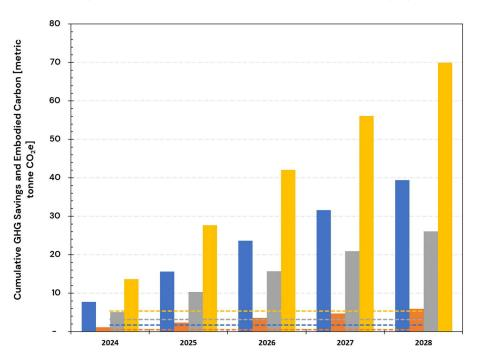
Figure A. 14: Embodied Carbon and Cumulative GHG Savings Over 5 Years (2024–2028) Using High RE Cost Electricity Emission Rates for CZ3 – Scenario 2: 100% Heat Pump Systems
