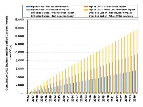
Figure A. 31: Embodied Carbon and Cumulative GHG Savings Over 75 Years (2024–2098) Using High RE Cost Electricity Emission Rates for CZ5 – Scenario 1: Natural Gas Heating
