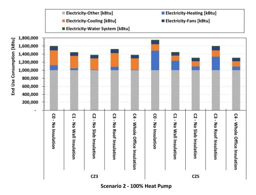
Figure 13: Electricity End Use Consumption for the Case with 100% Heat Pump Systems (Commercial Prototype)
