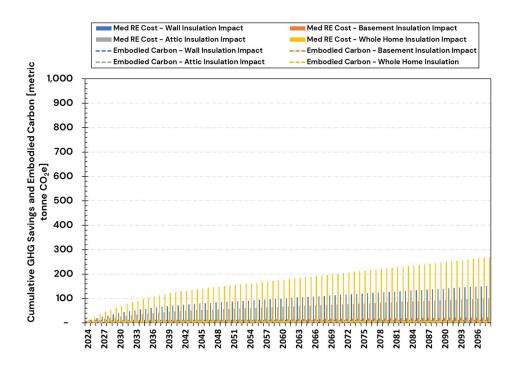
Figure A. 15: Embodied Carbon and Cumulative GHG Savings Over 75 Years (2024–2098) Using Medium RE Cost Electricity Emission Rates for CZ3 – Scenario 2: 100% Heat Pump Systems
