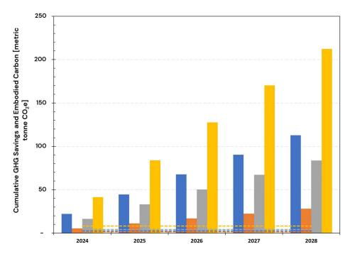
Figure A. 20: Embodied Carbon and Cumulative GHG Savings Over 5 Years (2024–2028) Using High RE Cost Electricity Emission Rates for CZ5 – Scenario 2: 100% Heat Pump Systems
