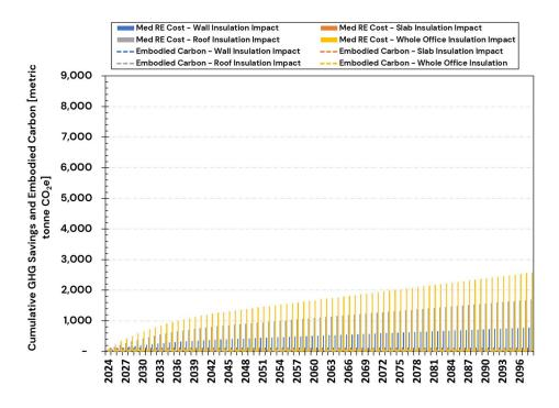
Figure A. 27: Embodied Carbon and Cumulative GHG Savings Over 75 Years (2024–2098) Using Medium RE Cost Electricity Emission Rates for CZ3 – Scenario 1: Natural Gas Heating
