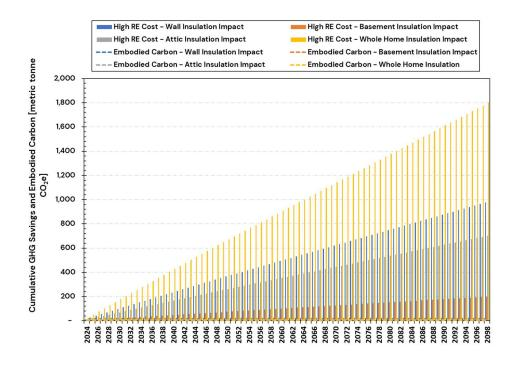
Figure A. 7: Embodied Carbon and Cumulative GHG Savings Over 75 Years (2024–2098) Using High RE Cost Electricity Emission Rates for CZ5 – Scenario 1: Current Heating Systems Mix
