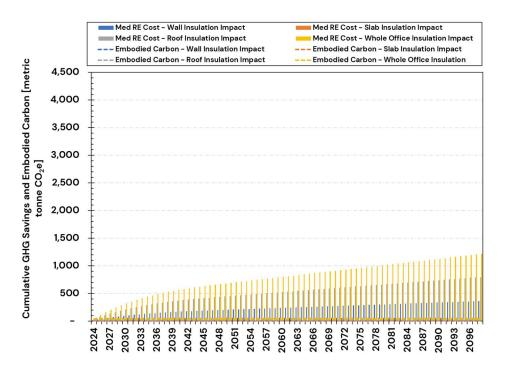
Figure A. 39: Embodied Carbon and Cumulative GHG Savings Over 75 Years (2024–2098) Using Medium RE Cost Electricity Emission Rates for CZ3 – Scenario 2: 100% Heat Pump Systems
