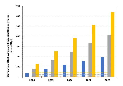
Figure A. 26: Embodied Carbon and Cumulative GHG Savings Over 5 Years (2024–2028) Using High RE Cost Electricity Emission Rates for CZ3 – Scenario 1: Natural Gas Heating
