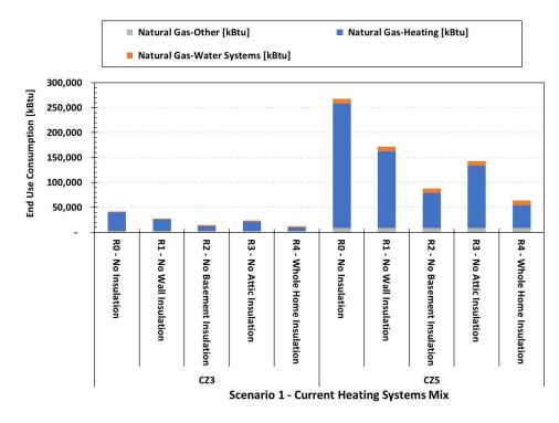
Figure 3: Natural Gas End Use Consumption for the Case with the Current Heating Systems Mix (residential)
