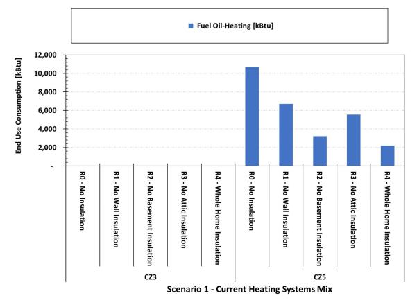
Figure 5: Fuel Oil End Use Consumption for the Case with the Current Heating Systems Mix
