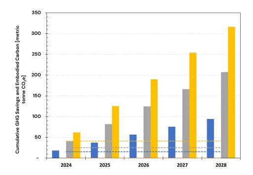
Figure A. 38: Embodied Carbon and Cumulative GHG Savings Over 5 Years (2024–2028) Using High RE Cost Electricity Emission Rates for CZ3 – Scenario 2: 100% Heat Pump Systems
