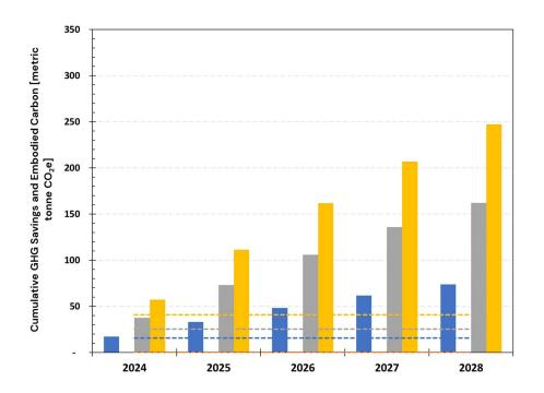
Figure A. 40: Embodied Carbon and Cumulative GHG Savings Over 5 Years (2024–2028) Using Medium RE Cost Electricity Emission Rates for CZ3 – Scenario 2: 100% Heat Pump Systems
