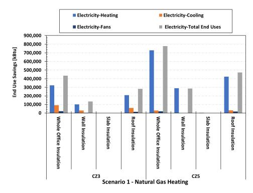
Figure 10: Impact of Insulation on Electricity End Use Percent Savings for Scenario 1 - Natural Gas Heating
