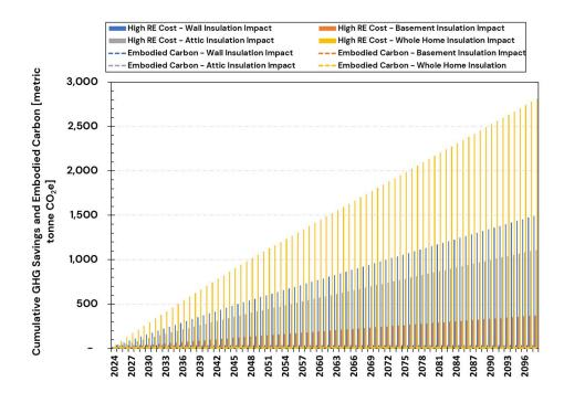
Figure A. 19: Embodied Carbon and Cumulative GHG Savings Over 75 Years (2024–2098) Using High RE Cost Electricity Emission Rates for CZ5 – Scenario 2: 100% Heat Pump Systems
