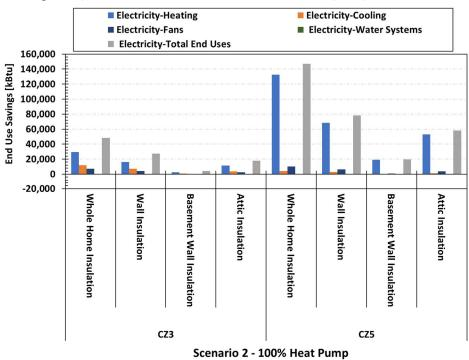
Figure 8: Impact of Insulation on Electricity End Use Savings for the Case with 100% Heat Pump Systems
