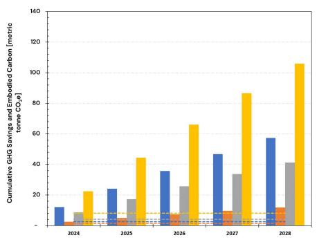
Figure A. 12: Embodied Carbon and Cumulative GHG Savings Over 5 Years (2024–2028) Using Low RE Cost Electricity Emission Rates for CZ5 – Scenario 1: Current Heating Systems Mix
