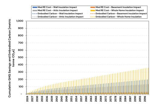
Figure A. 3: Embodied Carbon and Cumulative GHG Savings Over 75 Years (2024–2098) Using Medium RE Cost Electricity Emission Rates for CZ3 – Scenario 1: Current Heating Systems Mix
