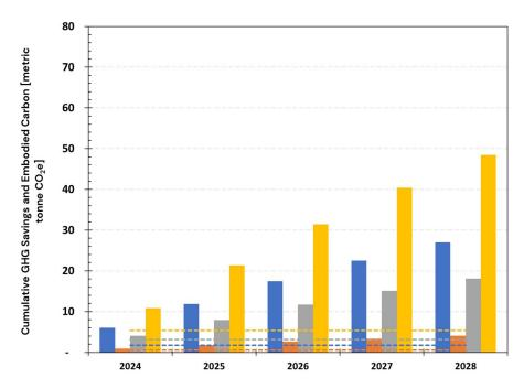
Figure A. 6: Embodied Carbon and Cumulative GHG Savings Over 5 Years (2024–2028) Using Low RE Cost Electricity Emission Rates for CZ3 – Scenario 1: Current Heating Systems Mix
