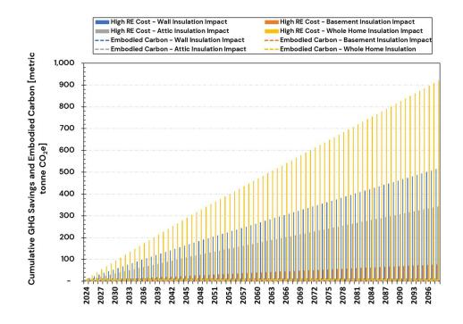
Figure A. 1: Embodied Carbon and Cumulative GHG Savings Over 75 Years (2024–2098) Using High RE Cost Electricity Emission Rates for CZ3 – Scenario 1: Current Heating Systems Mix
