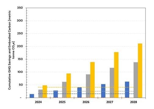
Figure A. 42: Embodied Carbon and Cumulative GHG Savings Over 5 Years (2024-2028) Using Low RE Cost Electricity Emission Rates for CZ3 – Scenario 2: 100% Heat Pump Systems
